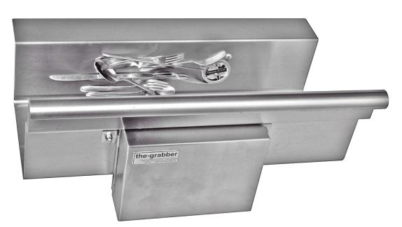
A focused magnetic retrieval system within a 16 gauge 300 series stainless steel water resistant sealed housing and mounting flanges. Each system consists of a pair, one **the-grabber** magnet unit mounted on each side of a trough. Model #G6915TEach6.75" x 9.75" x 1.75"For troughs up to 7.5" wide, 46#.\$1,500.00 ListModel #G6925TEach6.75" x 9.75" x 2.75"For troughs 7.5" to 9.5" wide, 64#\$1,750.00 ListModel #G6935TEach6.75" x 9.75" x 3.75"For troughs 9.5" to 12" wide, 92#.\$2,375.00 List
