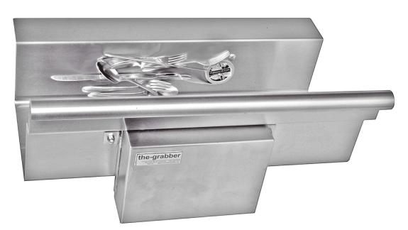
A focused magnetic retrieval system within a 16 gauge 300 series stainless steel water resistant sealed housing and mounting flanges. Each system consists of a pair, one **the-grabber** magnet unit mounted on each side of a trough.
